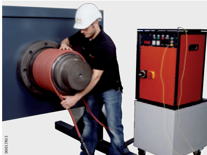
Figure 2 The flexible inductor can be wrapped around the component
