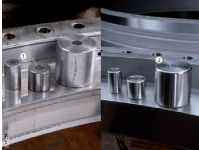
Figure 7 Rolling bearing raceway and rollers before and after reconditioning
