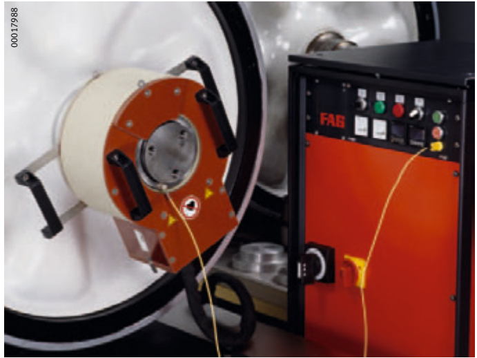
Figure 3 Rigid inductor in the dismounting of wheelset bearings
